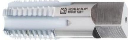
Interrupted Thread NPT Taper Pipe Taps have an odd number of lands, with every other tooth along the thread helix removed. The chamfer section is left with full threads to facilitate starting the tap. Interrupted Pipe taps allow better lubrication, free clearance of chips and requires less torque to drive. These taps are useful when used in tough metals or materials which load the cutting threads of the tap. Standard chamfer length is 2 - 3.1/2 threads.
