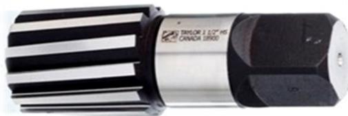
Taper Pipe Reamers are made for reaming holes to be tapped with American National Standard Taper Pipe Taps. They will prolong the life of any Taper Pipe Taps, as they ream the hole to the correct size and taper for tapping.
