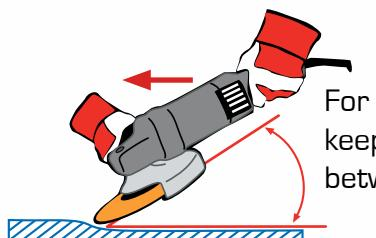
For fast stock removal, keep the grinding angle between 25° and 30°.
