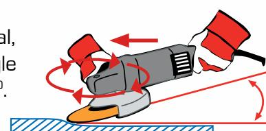
For finishing and blending, decrease the grinding angle to between 15° and 20°.
